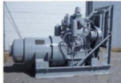
This is the heaviest duty 12.5 KW generator ever built combining the 2-71 Detroit Diesel engine with extremely heavy duty Delco or Emerson brushless alternators. The alternators are all copper wound and usually load test at over 15—20 KW.
