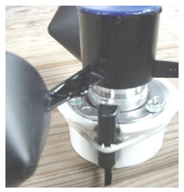
Completed anemometer hub assembly mounted in PVC reducer, with sensor attached
