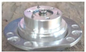
Nails in Motor for marking hub holes
